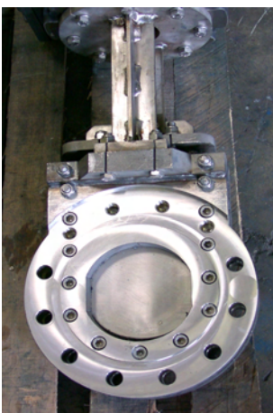
To the left, a 500 PSI 2 piece Split Body Fig 77 . This valve is constructed of all 316 Stainless Steel and has a one piece fully replaceable resilient seat . The valve is capable of bubble tight bi-directional shut off . The valve is also equipped with a 4:1 bevel gear operator. (Not shown)
